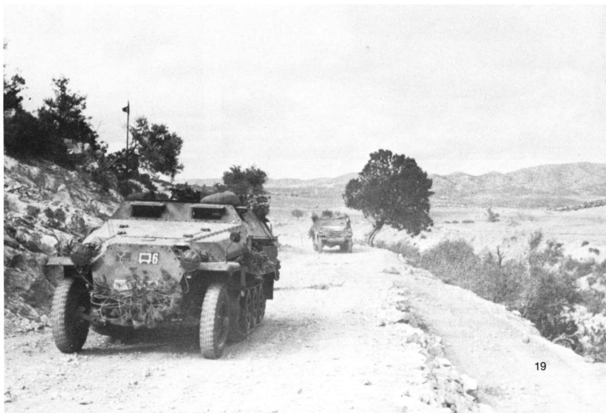
(Above Right) Ausf.Bs of the 8th Panzer Division, seen covered with branches. Track links are being carried on front, MG shields are fitted, and extra equipment is carried on the outside.
