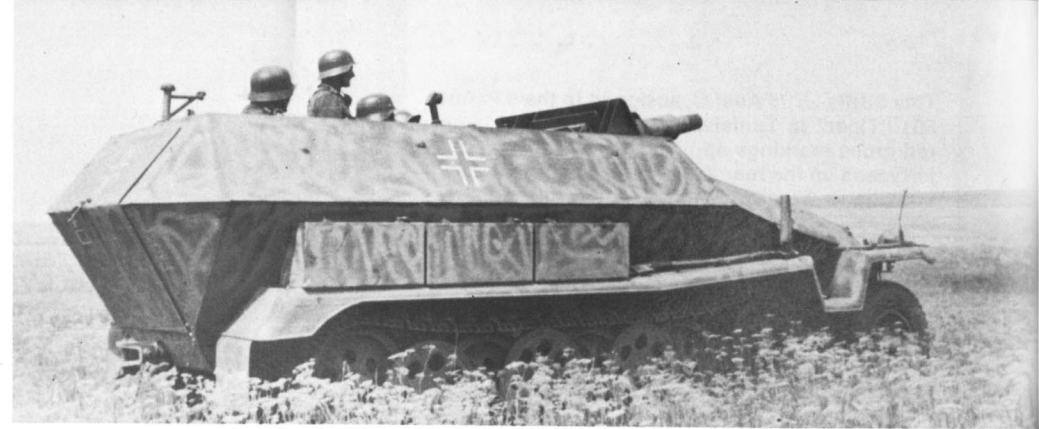
A SdKfz 251/9 Ausf.C in Russia, seen in the middle of 1943 in an elaborate camouflage pattern of dark Yellow over the old dark Gray. The gun telescope is clearly visible in front of the three soldiers. (Bundesarchiv)
