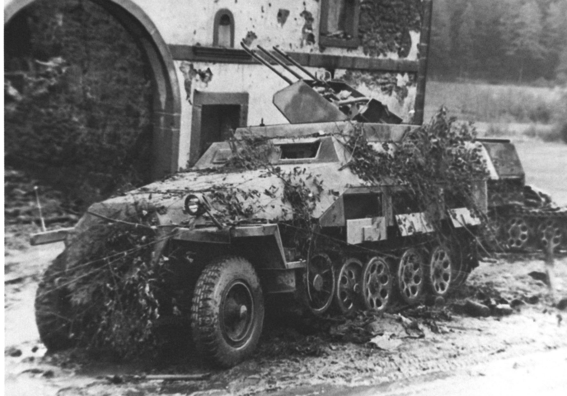
A field-modified SdKfz 251/21 based on the Ausf.C, the guns being fitted without the armor shield.
