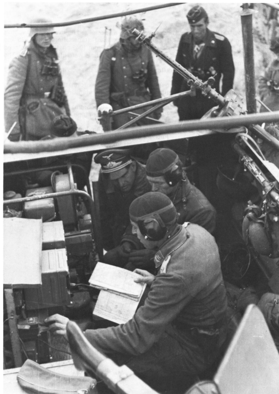
A view of the inside of the same vehicle with Luftwaffe personnel manning the FuG7 20 Watt transmitter. It is interesting that they are using the Luftwaffe MG 15 instead of the usual MG 34 for an air-defense weapon. (Bundesarchiv)
