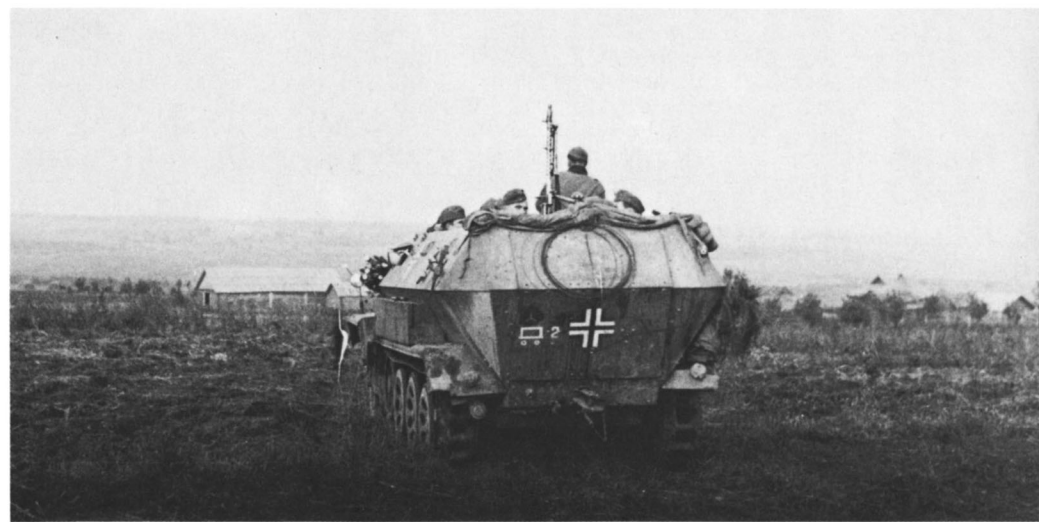
A rear view of an Ausf.A on the Northern Ost front in the Fall of 1941. The vehicle belongs to the 1st Panzer Division and is not fitted with an MG shield. Note the tactical sign on the rear plate, signifying motorized infantry. (Bundesarchiv)
