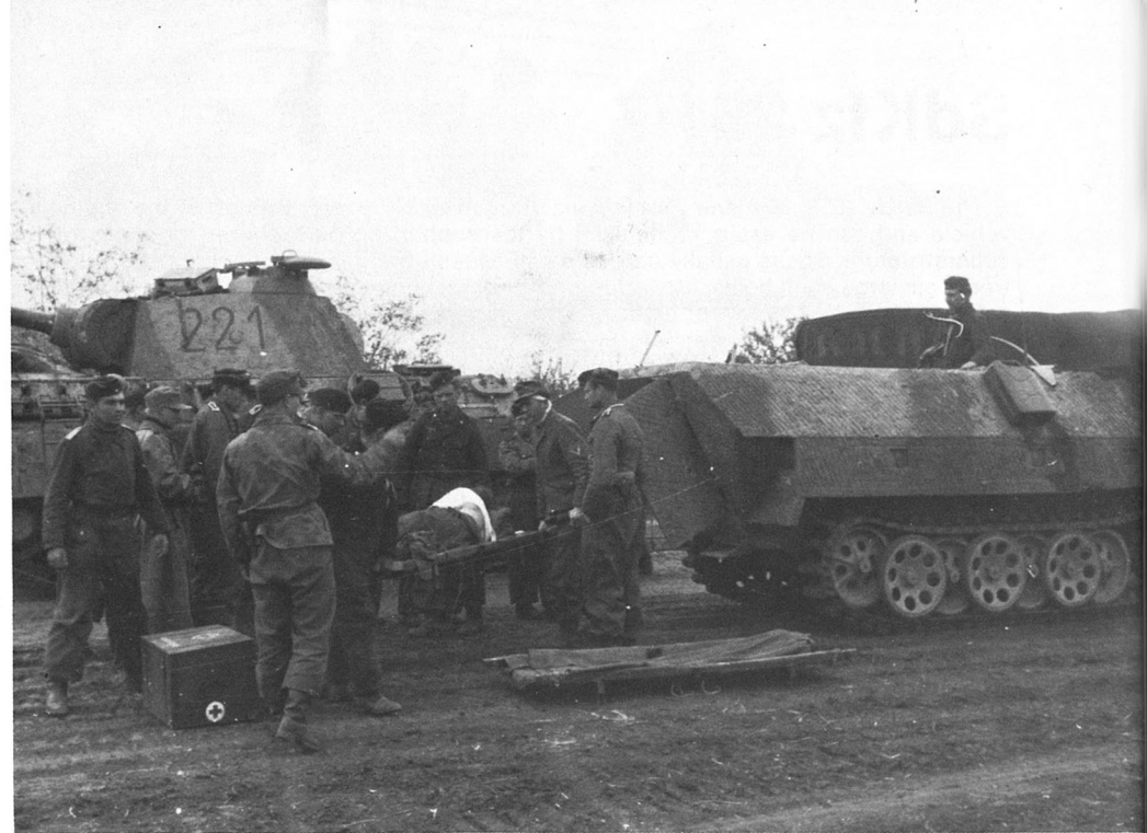
A SdKfz 251/8 Ausf.D, used for evacuation of wounded of a tank unit in the South of Russia in 1943. This vehicle has been coated with Zimmerit anti-magnetic paste, which is very unusual for an APC. (Bundesarchiv)
