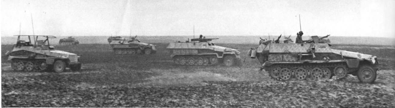
A combined battle-group — four SdKfz 251 Ausf.Cs, one SdKfz 251/10 mounting a 3.7 cm gun, a SdKfz 250/3 command vehicle and a PzKpfw II — on the open Russian steppe.
