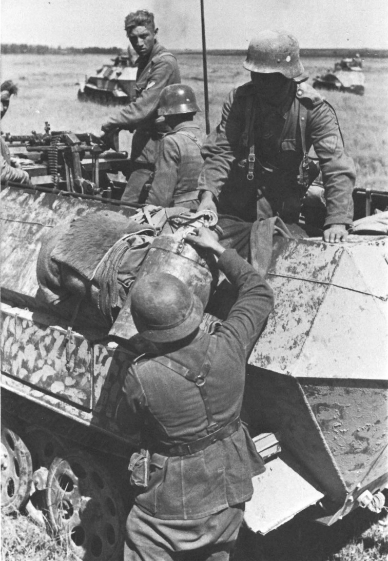
An Ausf.C of a heavy MG section. The front MG lacks the shield and is mounted on the heavy MG mount with a sighting telescope. Dried mud camouflage is clearly visible on this vehicle, Stalingrad, Fall, 1942. (Bundesarchiv)
