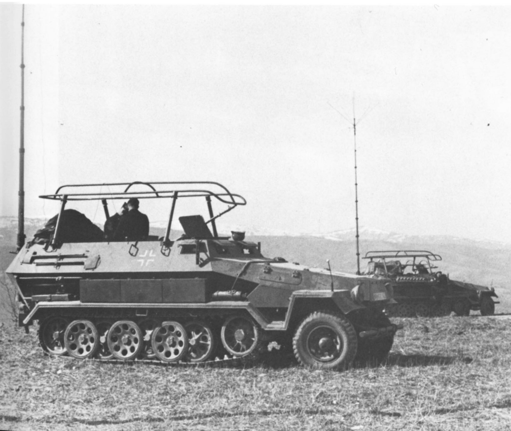
A SdKfz 251/3 I radio vehicle named Fuchs (Fox), in Russia. The frame aerial for the 30 Watt FuG8 transmitter was very conspicuous. (Bundesarchiv)
