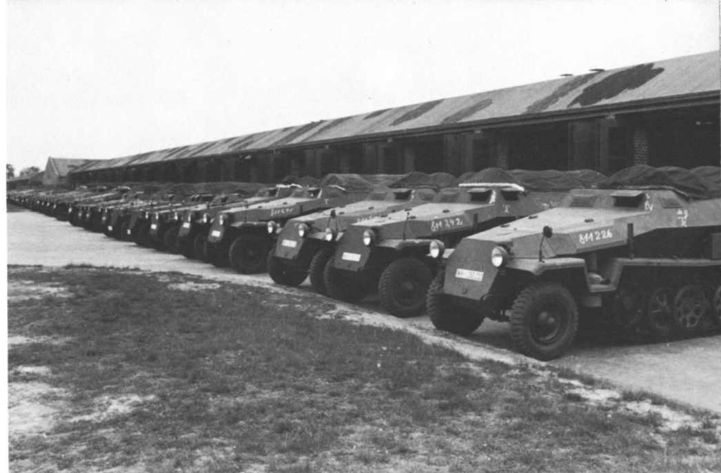
A group of brand new SdKfz 251 Ausf.Cs awaiting delivery to various units. Clearly distinguishable from the Ausf.A and B by the straight front plate, the vehicles carry chalk-on chassis numbers on the left intake cover. (Bundesarchiv)
