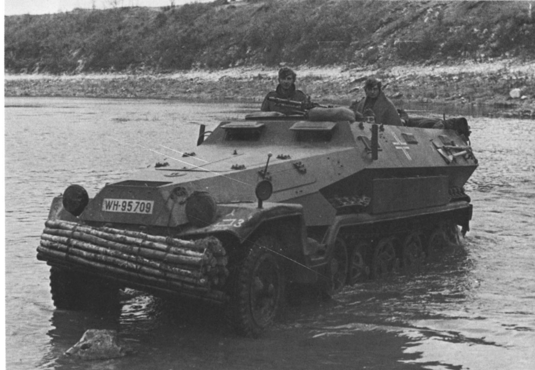
An early Ausf.A of the 1st Panzer Division, seen fording a river in Russia during the 1941 invasion. This vehicle is lacking the MG shield. The air intake at the top front of the engine compartment is clearly visible. The SdKfz 251 had a fording depth of up to 60 cm (2 feet). (Bundesarchiv)
