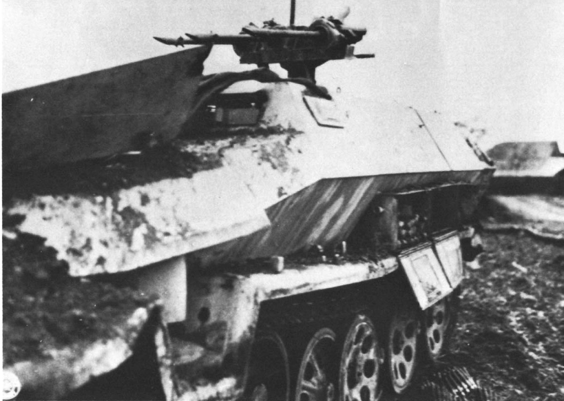
A field-modified SdKfz 251/21 based on the Ausf.C, the guns being fitted without the armor shield.
