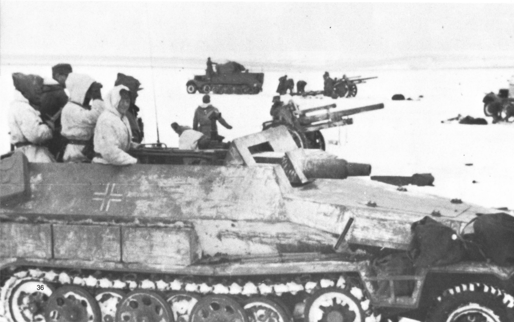
A SdKfz 251/9 Ausf.C in Russia, seen in the middle of 1943 in an elaborate camouflage pattern of dark Yellow over the old dark Gray. The gun telescope is clearly visible in front of the three soldiers. (Bundesarchiv)
