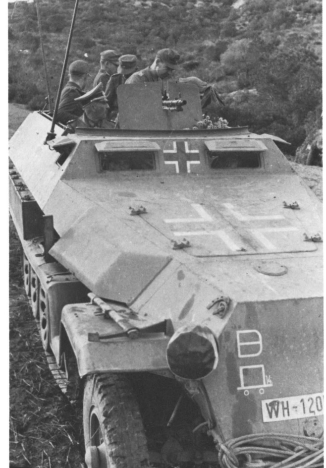
General Von Arnim's personal half-track in Tunisia, 1942. This Ausf.C belongs to the 21st Panzer Division and carries an additional cross on front plate between the visors and on the engine deck. (Bundesarchiv)
