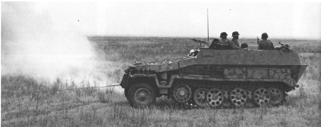
A disabled Ausf.C under tow shows a daubed mud camouflage pattern. This vehicle carries jerrycans on the front plate and the spare track links on the left fender.
