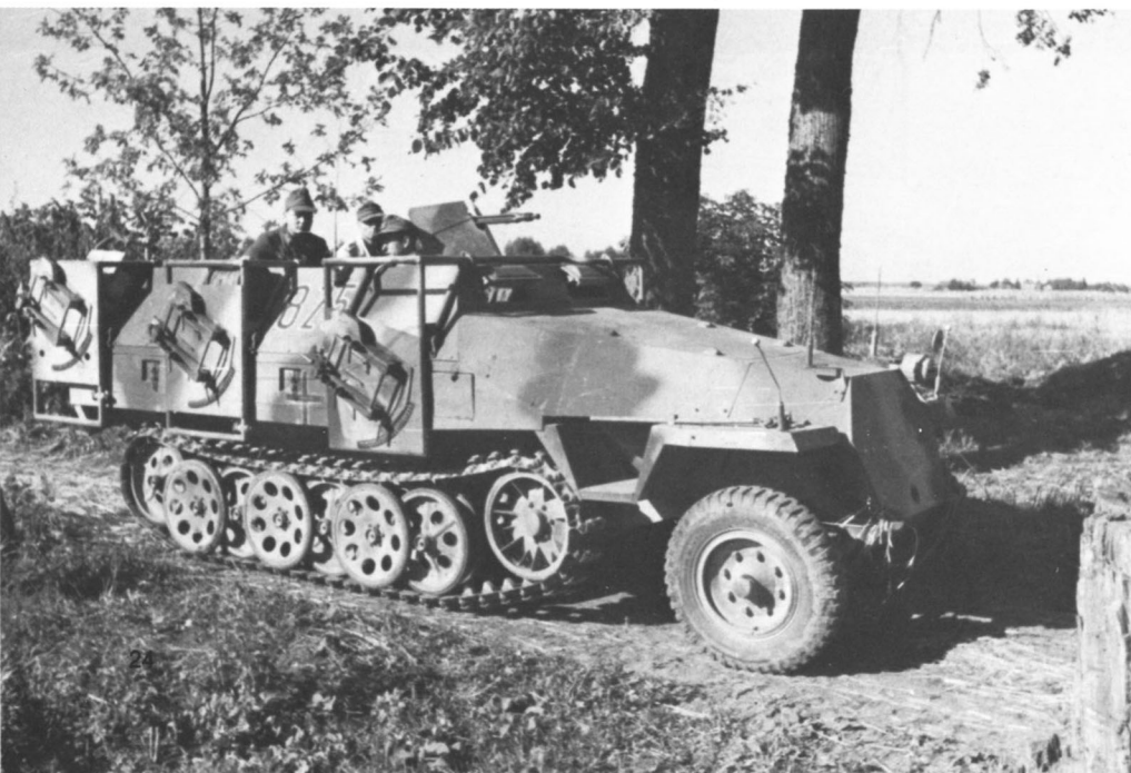
An Ausf.D with empty base plates on the Eastern Front during the Summer of 1944. This vehicle is sprayed in a three-tone camouflage pattern and carries a Red and White call number. (Bundesarchiv)
