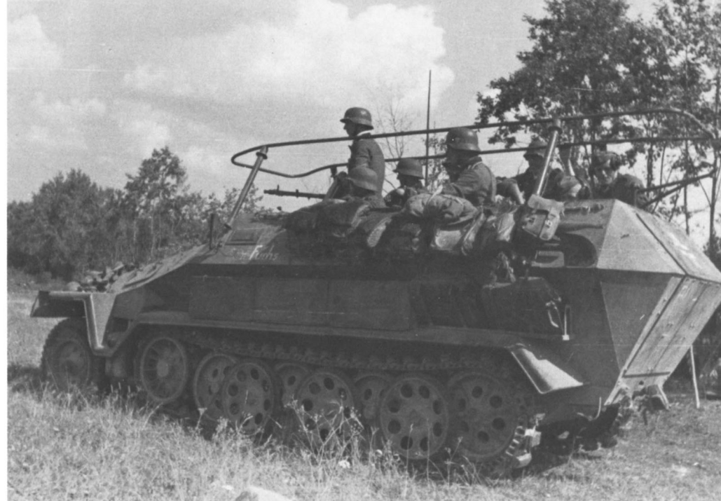
A SdKfz 251/3 I radio vehicle named Fuchs (Fox), in Russia. The frame aerial for the 30 Watt FuG8 transmitter was very conspicuous. (Bundesarchiv)
