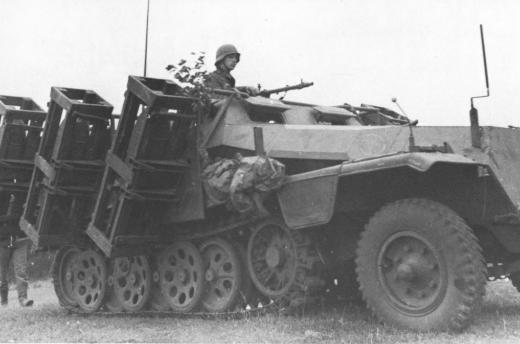
A fully loaded Ausf.C of the 24th Panzer Division in Russia, 1941. The rockets were stabilized in flight by spin rotation induced by the angled position of the rocket engine jets. (Bundesarchiv)
